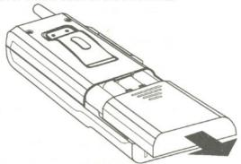
2. Insert 10 nickel cadmium batteries in the compartment.
